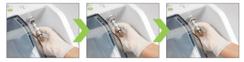
Assemble the adaptor connection on the maintenance attachment in the Assistina Twin
