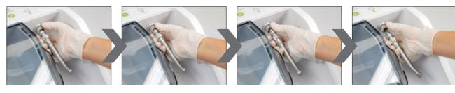
Remove the adaptor connection of the turbine handpiece from the maintenance attachment of the Assistina Twin
