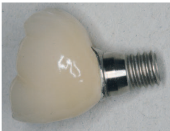
Fig. 1 Implant fracture after crestal bone loss. The geometry and the position of the external and internal threads were unfavourable.
