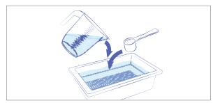
2. Place both water and powder into the instrument bath
